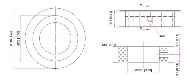
• 22 mm diameter pulley to be installed on the steering wheel for 10G potentiometer
