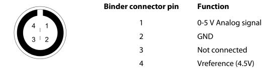
The steering potentiometer **electrical characteristics** are:
